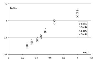
Fig. 9. Change of dimensionless constant of grinding  $K_1/K_m$  for greywacke
