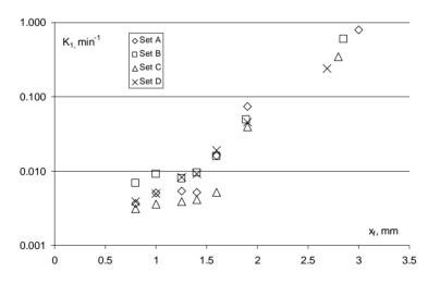
Fig. 5. Change of grinding constant value  $K_I$ , with feed granulometric composition after 30 minutes of grinding of quartzite for four ball sets
