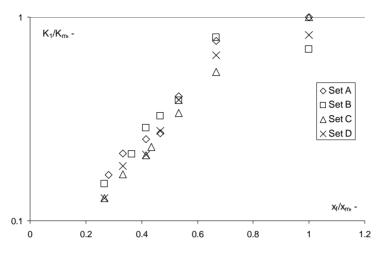
Fig. 10. Change of dimensionless constant of grinding  $K_{l}/K_{m}$  for granite
