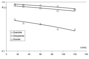
Fig. 3. Dependence between mass of the largest feed particle fraction and grinding time. Ball composition *C*
