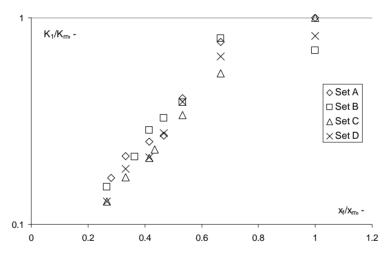
Fig. 7. Change of grinding constant value  $K_1$  and feed granulometric composition after 30 minutes of grinding of granite for four ball sets
