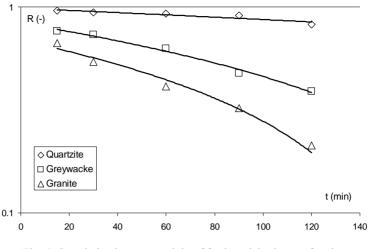
Fig. 4. Correlation between weight of feed particles largest fraction and grinding time. Balls composition D
