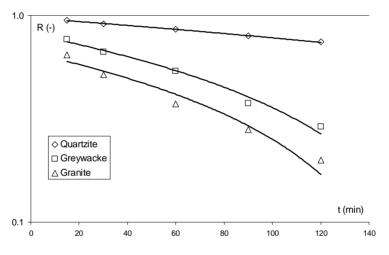
Fig. 1. Dependence between mass of the largest feed particle fraction and grinding time. Ball composition A
