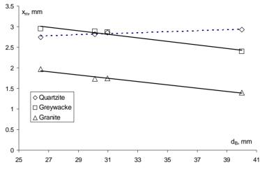
Fig. 11. Correlation between optimum feed size  $x_m$  and ball diameter  $d_B$
