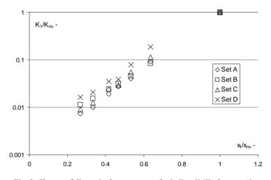
Fig. 8. Change of dimensionless constant of grinding  $K_1/K_m$  for quartzite
